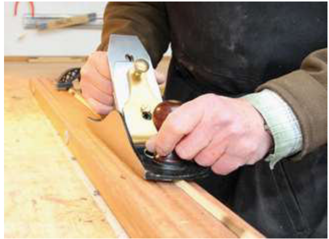
Wooden Rough Planing Form with 60 Degree Gauges in different sizes. à Note the big Plane.
