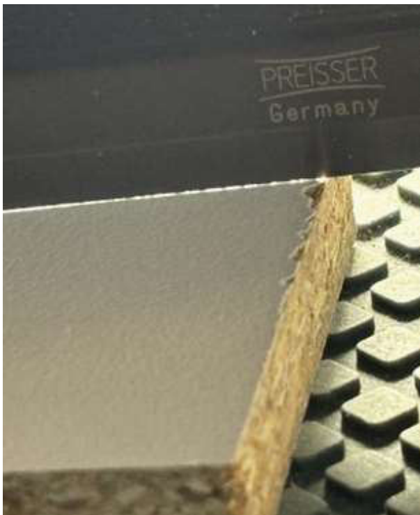
In fig. 1.1 The light thread is extremely thin and granular due to the embossing of the surface. Embossing which is very useful because if you see it, it means that the blade is exactly flush, that is, it only touches the peaks of the embossing. An excellent way to establish zero.
