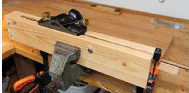
Device to hold the Blank at an Angle for Planing Splices
