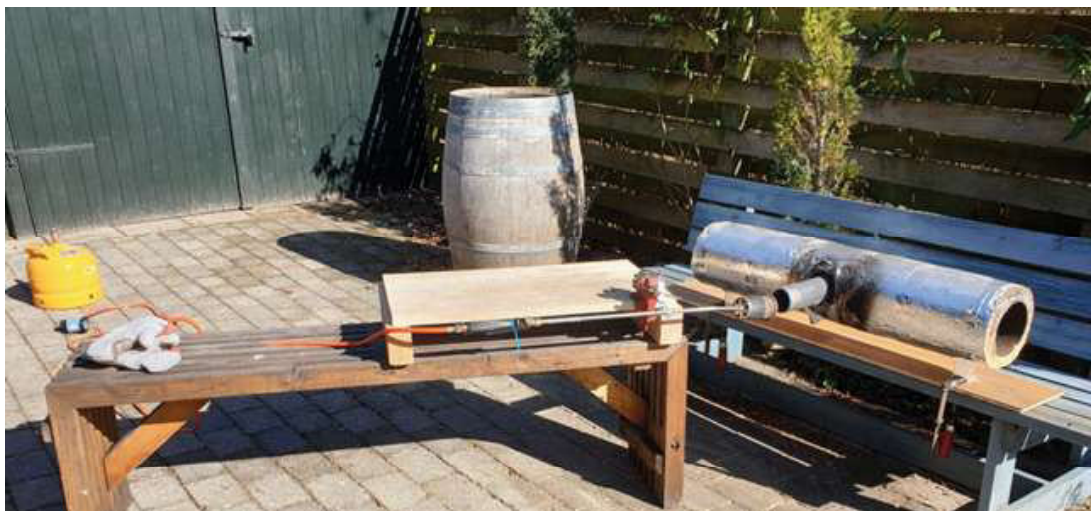
Heat Treating "oven" and Gas Burner Set Up
