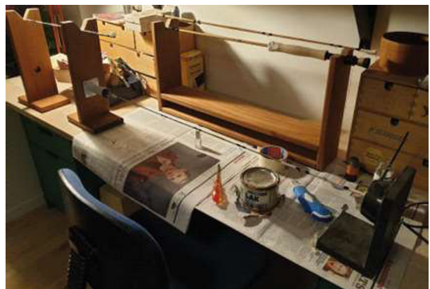
Varnishing Guide Wraps while turning the Blank slowly with a Grill Motor/ Ball Bearing Set Up.
